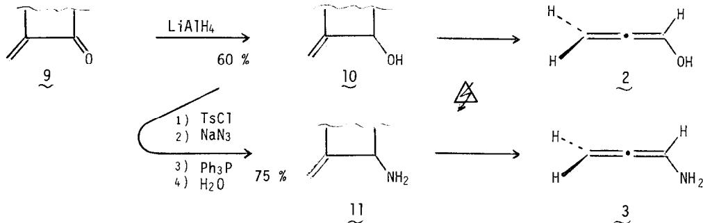
Thermolysis of alcohol 10 (760°C, 10<sup>-5</sup> torr) leads, besides a small amount of acrolein, to propadienol 2 (45 %) ; m/e (70 eV) : 56 ( $\text{M}^+$ , base peak) ; δ<sup>1</sup>H (CFCl<sub>3</sub>, -90°C) : 5.30 (d, 6 Hz, 2H) - 6.56 (dt, 6 and 10 Hz, 1H) - 7.00 (d, 10 Hz, OH) ; ir (solid, -196°C) : 1980 - 1960 (C=C=C, broad). By warming up to -50°C, 2 tautomerizes quantitatively into acrolein.
